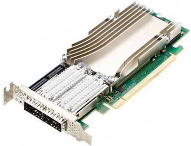
Fig. 1. The FPGA based NFB-200G2QL acceleration card.
